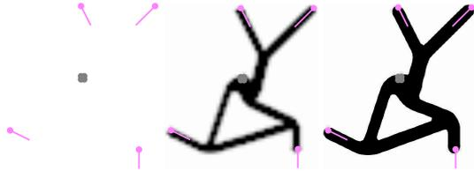
**Figure 8:** Chassis synthesis by topology optimization. **Left:** four forces resulting from hinges at a given time frame (pink) and attachment point (gray). **Middle:** Optimized densities for these forces. **Right:** Final shape after smoothing and contour extraction.
