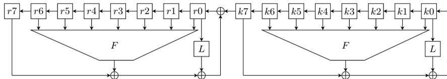
**Fig. 4.** One round of the ESSENCE hash function. The chaining value  $CV$  is loaded into the  $r_i$  registers, whereas the message  $M$  is loaded into the  $k_i$  registers. Every register is either 32 or 64 bits, resulting in a hash value of either 256 or 512 bits. Function  $F$  is a bitwise non-linear function, and  $L$  is a linear function operating on an entire word. ESSENCE consists of 32 rounds, after which a feed-forward is applied.
