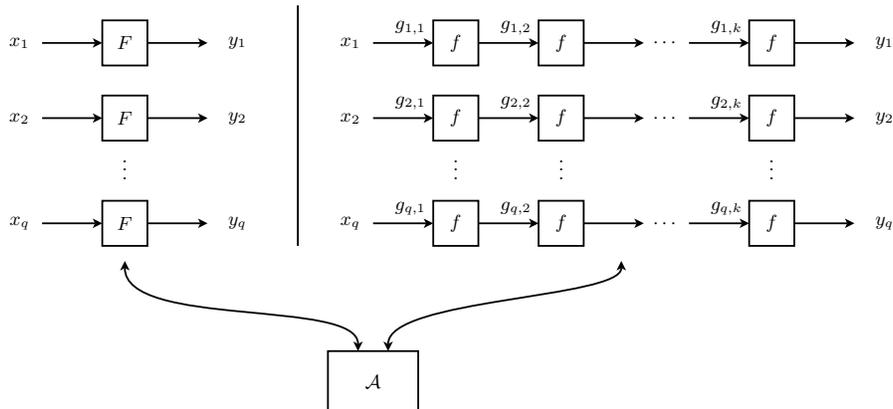
**Fig. 1.** Distinguishing between a random function (resp. permutation)  $F$  and a random function (resp. permutation)  $f$  that is iterated  $k$  times. The adversary  $\mathcal{A}$  makes at most  $q$  queries. All queries are assumed to be distinct. In case  $F$  and  $f$  are permutations, the  $\mathcal{A}$  can make both forward and inverse queries.
