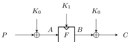
**Fig. 5.** The PRIDE block cipher, which processes 64-bit plaintext  $P$  using a 128-bit key  $K$ , which is split into two 64-bit keys  $K_0$  and  $K_1$ . Key  $K_0$  is used for prewhitening and postwhitening. The block cipher  $F$  is a 20-round Substitution-Permutation Network (SPN) that uses  $K_1$ .
