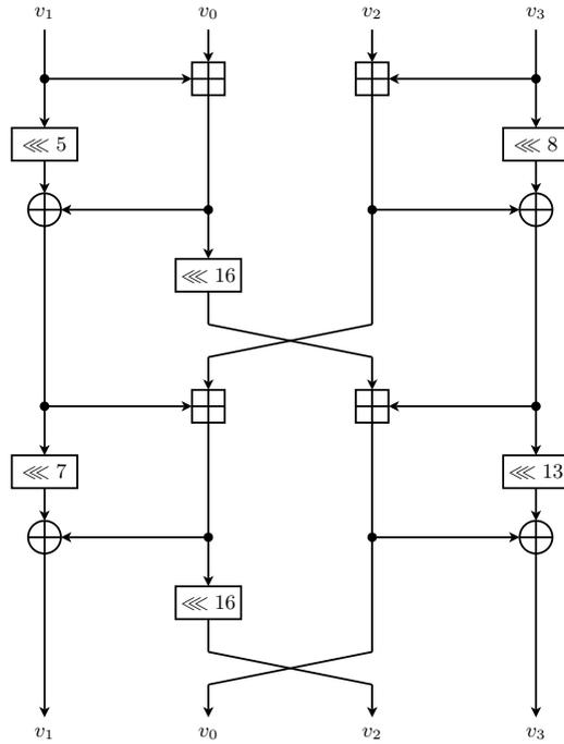
**Fig. 2.** One round of the Chaskey permutation  $\pi$ , defined as:  $v_0\|v_1\|v_2\|v_3 \leftarrow \pi(v_0\|v_1\|v_2\|v_3)$ . The values  $v_0$  and  $v_1$  are intentionally swapped, as this reduces the number of crossing lines in the figure.
