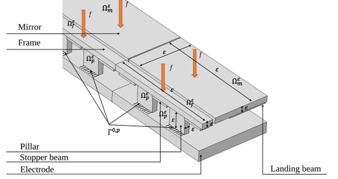
Fig. 11: Scales and heat loads on a cell
