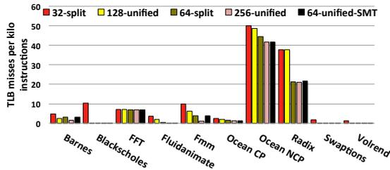
Figure 11: TLB misses per thousand instructions for split or unified TLBs on  $4W \times 4T$  DITVA
