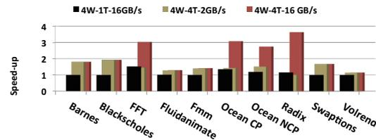
Figure 12: Performance scaling with memory bandwidth, relative to 4-thread SMT with 2 GB/s DRAM bandwidth
