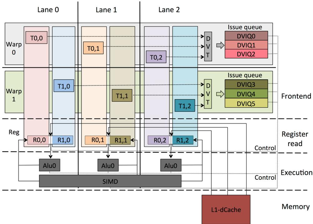
Figure 2: A logical view of the DITVA architecture
