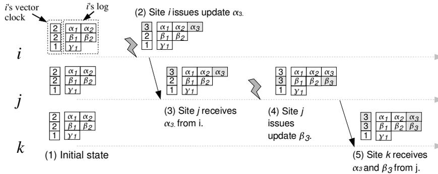
Fig. 16. Example of operation propagation using vector clocks. Symbols α, β and γ show updates submitted at *i*, *j*, and *k*, respectively. Shaded rectangles show changes at each step.
