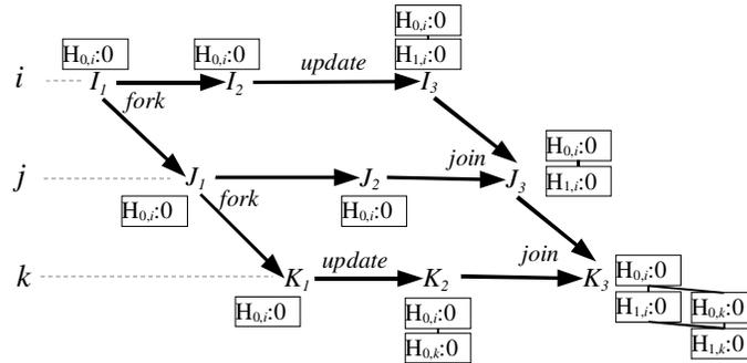
Fig. 14. Example of the use of hash histories (HHs) using the same scenario as Figure 13. The object starts as a single replica on  $i$  with a HH of  $H_0$ , where  $H_0$  is a hash of the current contents of the object. After an update at  $i$ , the HH becomes  $H_0$ - $H_1$  by appending the new contents hash. The result of merging and resolving two conflicting updates ( $K_3$ ) is represented in the HH by creating an acyclic graph as shown.
