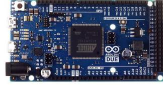
Fig. 2. The Arduino DUE microcontroller based board
