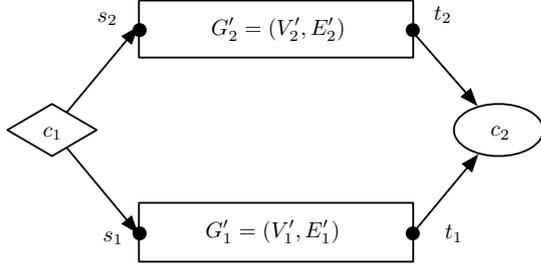
Fig. 1. A canonical conditional construct with branching factor 2. Vertices  $s_1$  and  $t_1$  (vertices  $s_2$  and  $t_2$ , resp.) are the sole source vertex and sink vertex of  $G'_1$  ( $G'_2$ , resp.).
