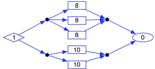
Fig. 4. The DAG  $G_i$  of an example conditional DAG task  $\tau_i$ . For this task,  $D_i = 15$  and  $T_i = 20$ . Note that  $len_i = 11$  and corresponds to taking the lower branch of the conditional, while  $vol_i = 25$  and corresponds to taking the upper branch.
