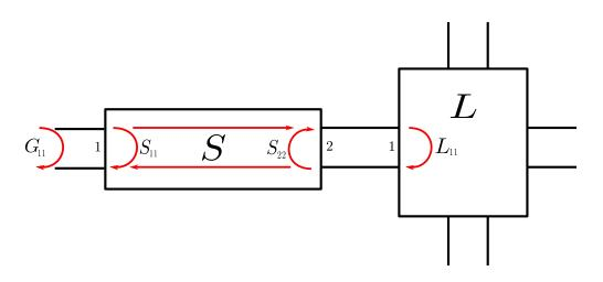
Figure 1: Filter plugged to a load L with reflexion coefficient  $L_{11}$
