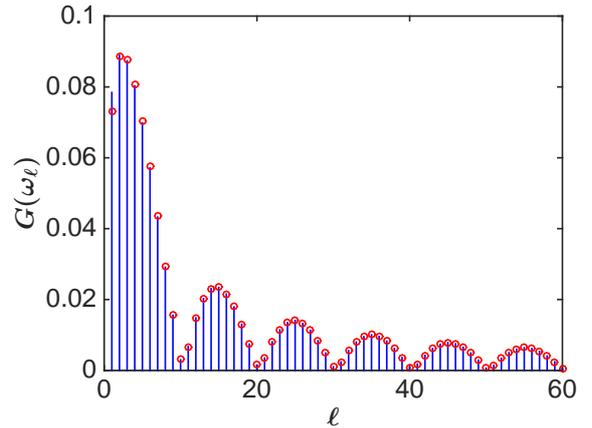
FIG. 3. (Color online) MI gain for  $\omega = \omega_\ell$  as a function of  $\ell$ ; Red circles, estimated gain given by (20). Parameter values are  $\beta_{av} = 1$ ,  $Z = 1$ ,  $\gamma_{av} = 1$ ,  $P = 1$ ,  $\beta_m = 0.1$ .
