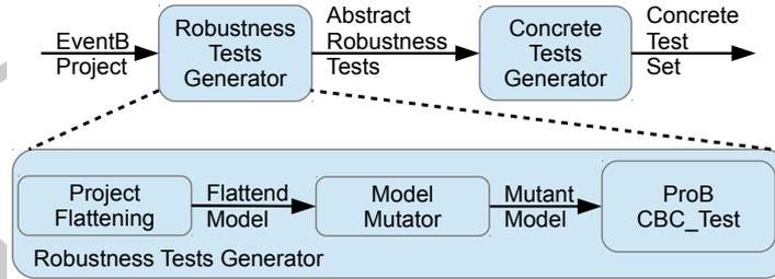
Fig. 1. Overview of the Robustness Test Generation Process
