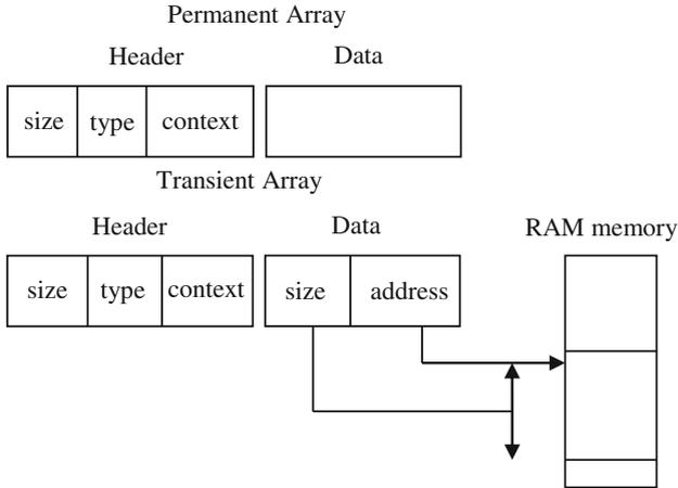
**Fig. 1.** Structure of transient and permanent arrays.
