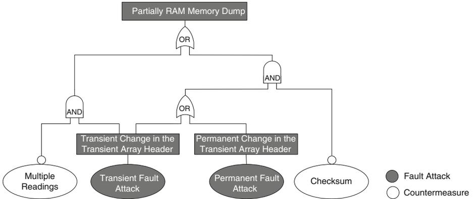
**Fig. 2.** Fault tree overview of the different possible attack paths to fulfill a partial memory dump of the RAM by a fault attack. Furthermore, effective countermeasures against the two general types of fault attacks are listed.
