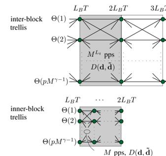
FIG. 2: Simplified detection with  $k = 1$  (pps-paths per state).
