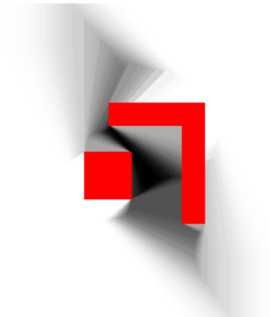
Fig. 19. Definition based on dilation by a structuring element derived from the angle histogram, with Equation 17.
