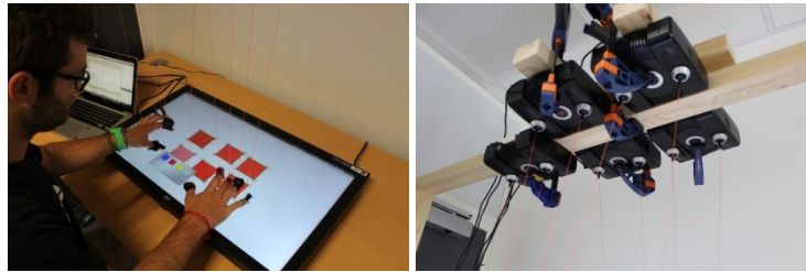
Fig. 3: Experimental setup: (left) participant completing TASK T1 using the Finger Palette ; (right) the 5 GameTrak devices located above the 32" 3M touchscreen.
