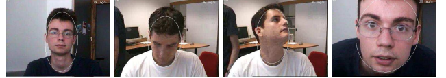
Figure 1: Example of face tracking. First and second moments provides an ellipse which delimit the face in the image
