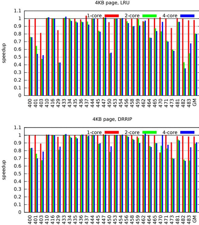
**Figure 3: Impact of replacing the baseline L3 replacement policy with LRU (upper graph) and with DRRIP (lower graph). Performance is relative to baselines for 4KB pages. The rightmost cluster of each graph is the geometric mean over the 29 benchmarks.**
