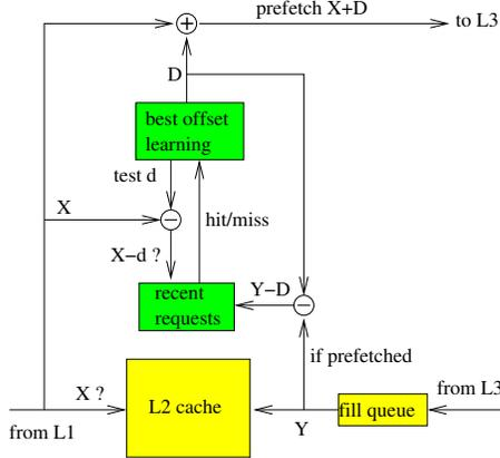
Figure 1: Schematic view of a BO prefetcher.
