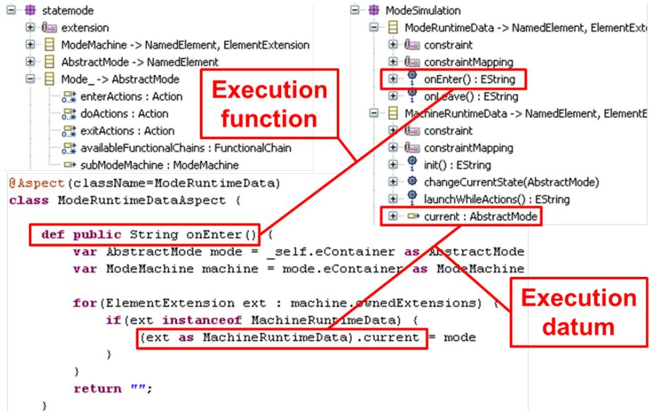
Fig. 2. GEMOC-xCapella: Definition of execution functions and data
