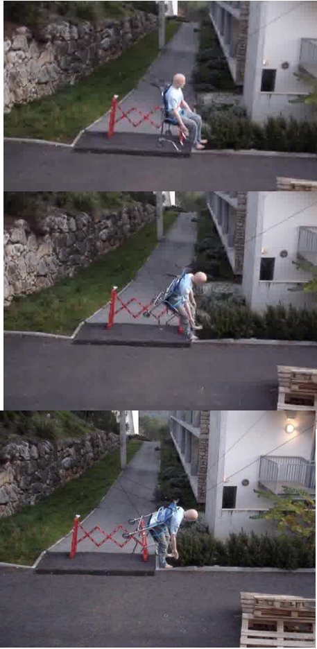
Fig. 3. An experiment showing changes of cable configuration for an infinitesimal change in the cable lengths leading to very different poses
