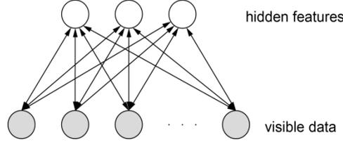
**Figure 2:** Network Structure of a Restricted Boltzmann Machine
