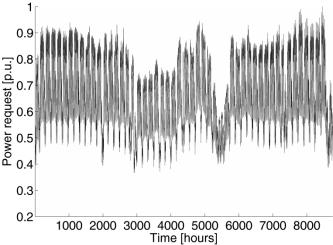
Fig. 3. Chronological Load Curve for direct MV customers.
