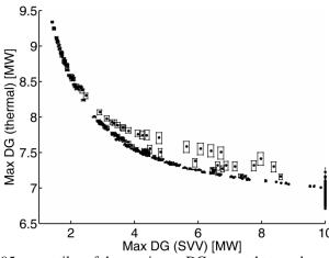
Fig. 9. Rectangles of the 0.05 and 0.95 percentiles of the maximum DG power that can be connected to all the buses in their most limiting time band, with respect to Supply Voltage Variations and thermal limits. Each rectangle corresponds to a bus. Dots mark the DLF results.
