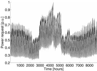
Fig. 4. Chronological Load Curve for MV/LV transformers.
