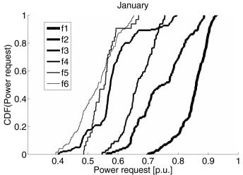
Fig. 5. The cumulative power request probability distributions of the six time bands of January for direct MV customers. These distributions are built from the chronological load curves of January (Fig. 3).
