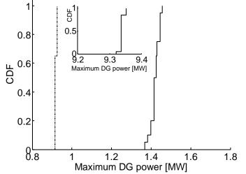
Fig. 8. The probability of SVV (solid line), Rapid Voltage Changes (dashed line), and LTL (inset) constraint violation as a function of the maximum DG connected to bus 48 in the most limiting time band, i.e., April – f5. The CDFs quantify the probability to violate the constraints during April – f5 if a given amount of power is generated at bus 48.
