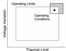
Fig. 1. Abstract representation of the 2D phase space of the electrical network. For clarity but with no loss of generality, only two dimensions are shown.
