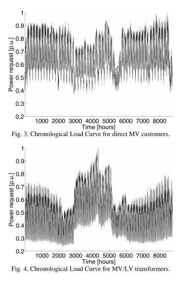
These curves have been derived from the data made available by the Italian Transmission System Operator (TSO), Terna, which represent the demand profiles of the two different MV load classes on a national basis. Given that the two loads' classes use energy at different rates during time, it is necessary to model the relevant power absorption by two different load curves.
