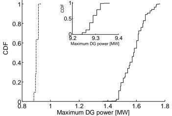
Fig. 7. The yearly probability of SVV (solid line), Rapid Voltage Changes (dashed line), and LTL (inset) constraint violation as a function of the maximum DG connected to bus 48. The CDFs quantify the yearly probability to violate the constraints if a certain amount of power is generated at bus 48.
