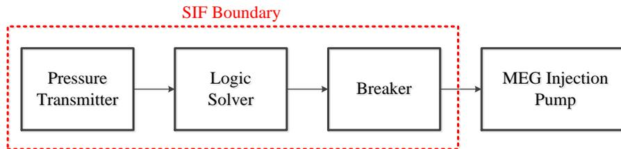
Figure 7. MEG Subsea Injection Pump PSHH Configuration
