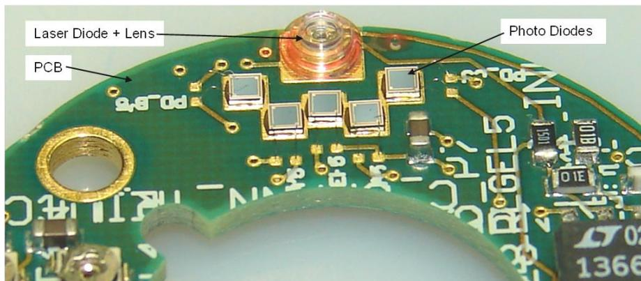
**Fig. 6.** Complete assembled optic module on PCB
