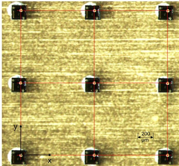
**Fig. 3.** 3x3 Laser diode array on PCB
