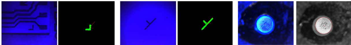
Fig. 6: Samples of reference marks with corresponding results from image-processing (from [4]).
