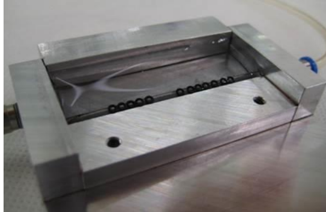
Fig. 5. Arranged components in a row after vibration
