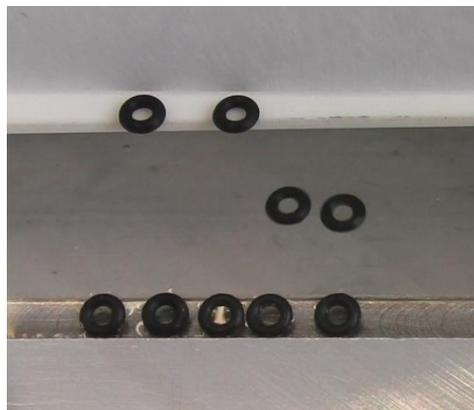
Fig. 2. Sliding o-rings on a convex fluidic surface
