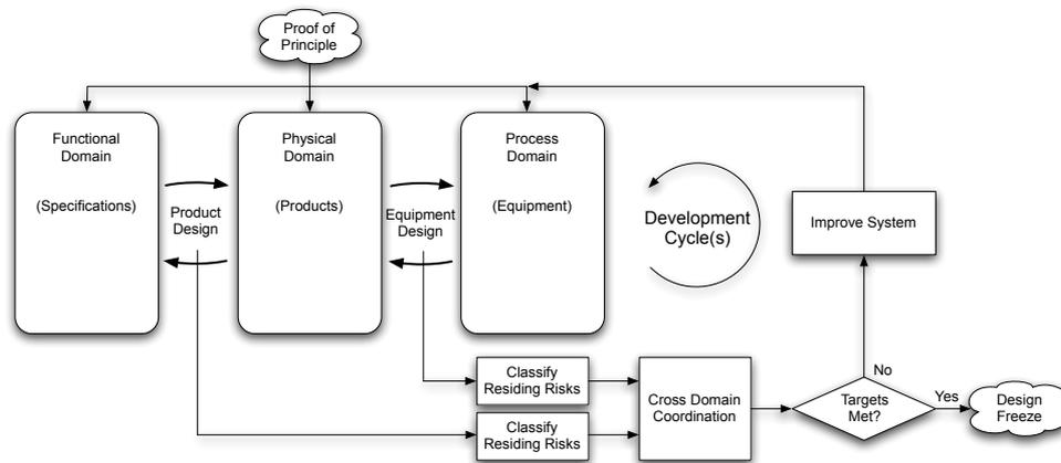
**Fig. 4** Multi Domain Development Cycle for cross-domain coordination. The risk classification results from product design and equipment engineering processes are taken into general consideration. Joint classification if targets are met and what to do to fulfil them in the next cycle are point of discussion before definition of improvements. Struggles for engineers are administered and equally divided
