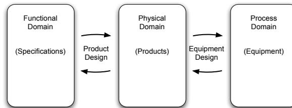
**Fig. 2** Relational mapping of the domains. Specifications in the functional domain are brought into relation to design parameters of a product in the physical domain by the product design process. The design parameters are related to the process domain by the equipment design process
