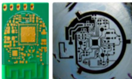
**Fig. 5** Left, printed circuit board of a wireless sensor system.
