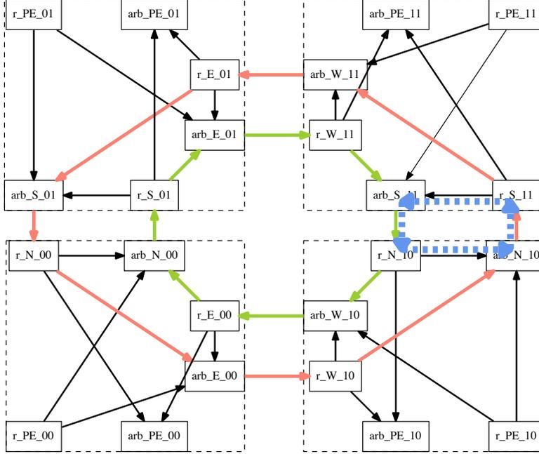
Figure 6: Illustration of the two circular paths that a packet can reach any node and the livelock loop  $r\_N_{10} \rightarrow arb\_N_{10} \rightarrow r\_S_{11} \rightarrow arb\_S_{11} \rightarrow r\_N_{10}$ .
