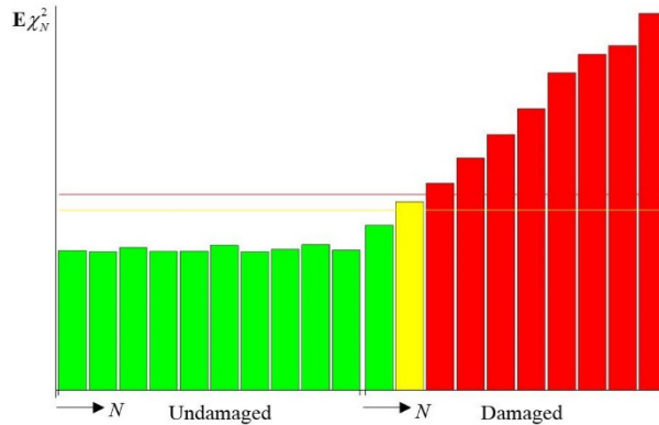
Fig 2 Expected \chi_N^2 value evaluated for different number of samples in damaged and undamaged conditions (red line: 99 percentile, yellow line: 95 percentile)
