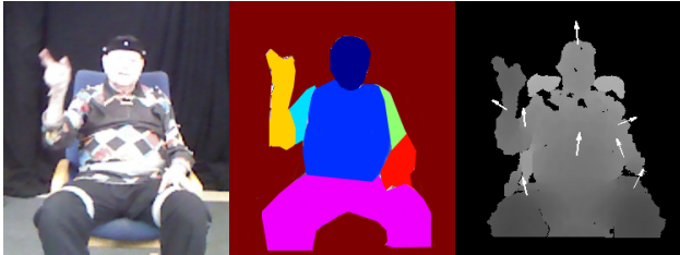
Figure 2. Human-limb segmentations, alongside depth, can be exploited to fit surfaces corresponding to parts of the body. Normals to these surfaces can then be estimated, and these normals give an indication of the stability of the user’s pose. In the event of the user being in an unstable pose, the robot can use knowledge of these normals to help the user gain a stable pose by exerting the necessary physical force in the optimal direction.
