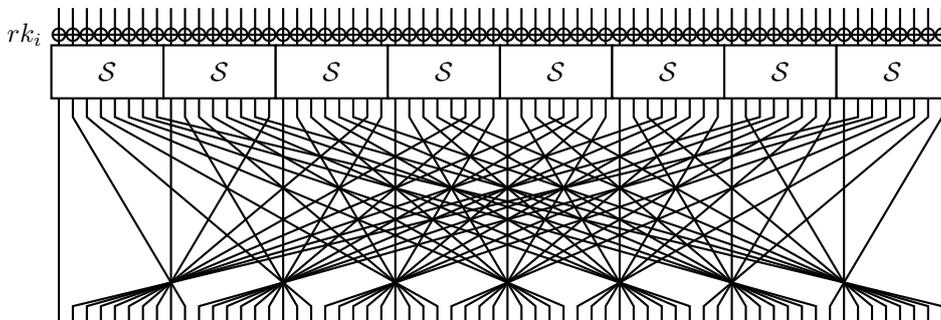
Figure 5.1: The round function of FLY. Bits are numbered left to right from 0 to 63 (w.r.t. the bit permutation). The addition of the round constant is omitted.
