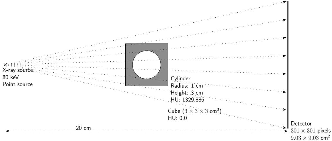
**Figure 13:** Simulation setup.
