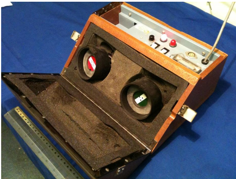
Fig 1: An acoustic coupler and modem – the telephone handset rested on the two cups to transmit and receive digital data encoded as sound frequencies
