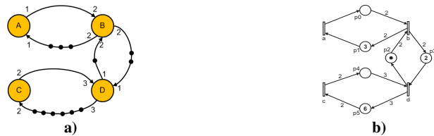
Fig. 1. An example of a Dataflow model, where some arcs contain initial tokens (a) and Petri net model (b).
