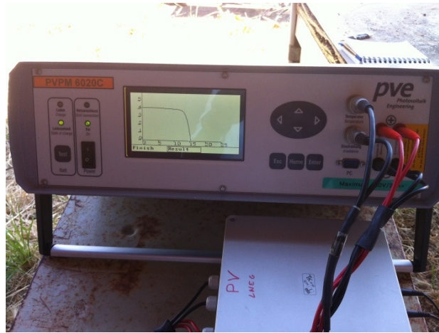
Fig. 2. Experimental I-V curves.
