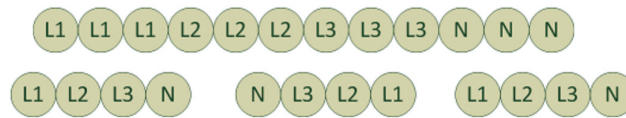
Fig. 6. Present arrangement (top) and proposed re-arrangement (bottom) of cables connecting the transformer and the main switchboard.
