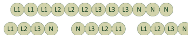
Fig. 6. Present arrangement (top) and proposed re-arrangement (bottom) of cables connecting the transformer and the main switchboard.
