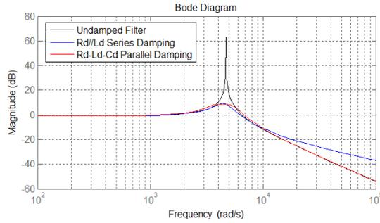
Fig. 4. Magnitude bode plot of the LCL filter
