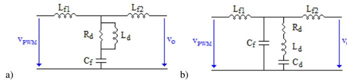
**Fig. 3.** Practical approaches to the damping of the LCL filter: a) Parallel  $R_d$  and  $L_d$  in series with the shunt capacitor. b) Series  $R_d$ ,  $L_d$  and  $C_d$  in parallel with the shunt capacitor
