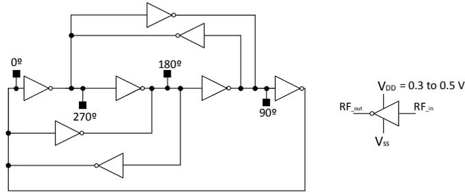
Fig. 4. Quadrature four-stage ring oscillator.
