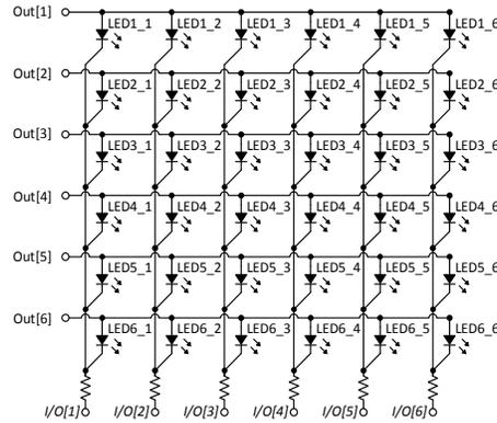
Fig. 4. Example model of an LED matrix.
