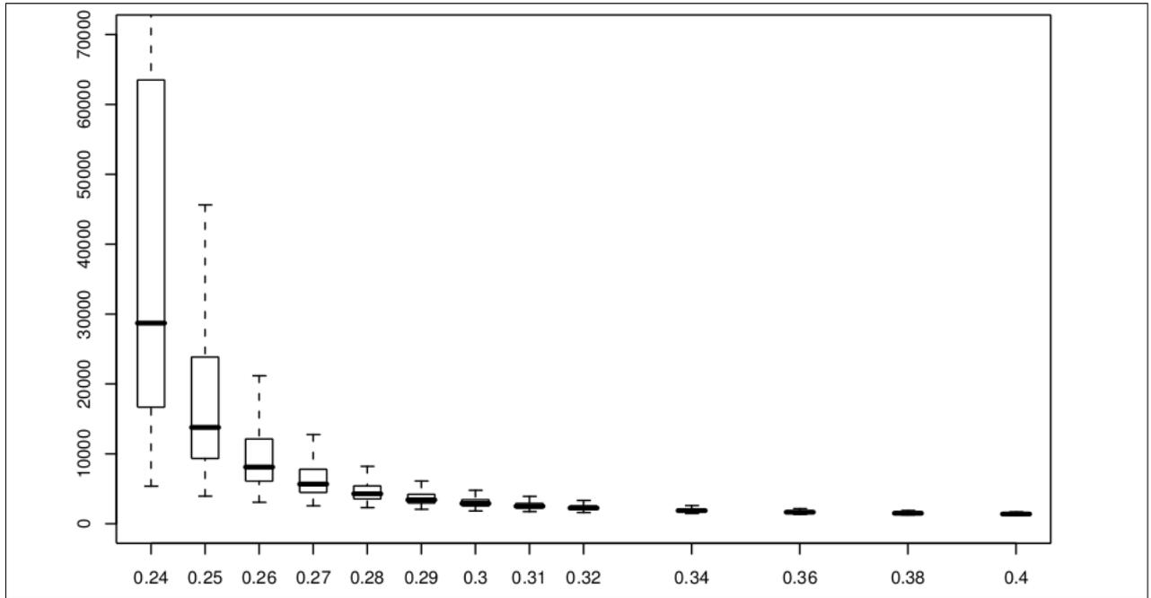
**Fig. 1:** Boxplot for total number of keys examined by Heninger and Shacham algorithm for 2048 – bit N, varying  $\delta$ . This figure has been taken from [HS09] and is given here to show that our results closely match those of [HS09] as also suggested by our theoretical analysis.
