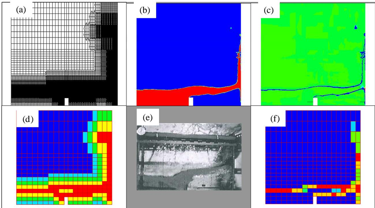
FIG. 3 – Dambreak with block remeshing at  $t=0.4s$ . (a) Mesh; (b) Density (air-blue, water-red); (c) Density of numerical entropy production (equation (2)): green-zero, blue-negative values); (d) Mesh refinement level per block (1 to 5); (e) Experiment [16]; (f) Mesh refinement criterion per block.
