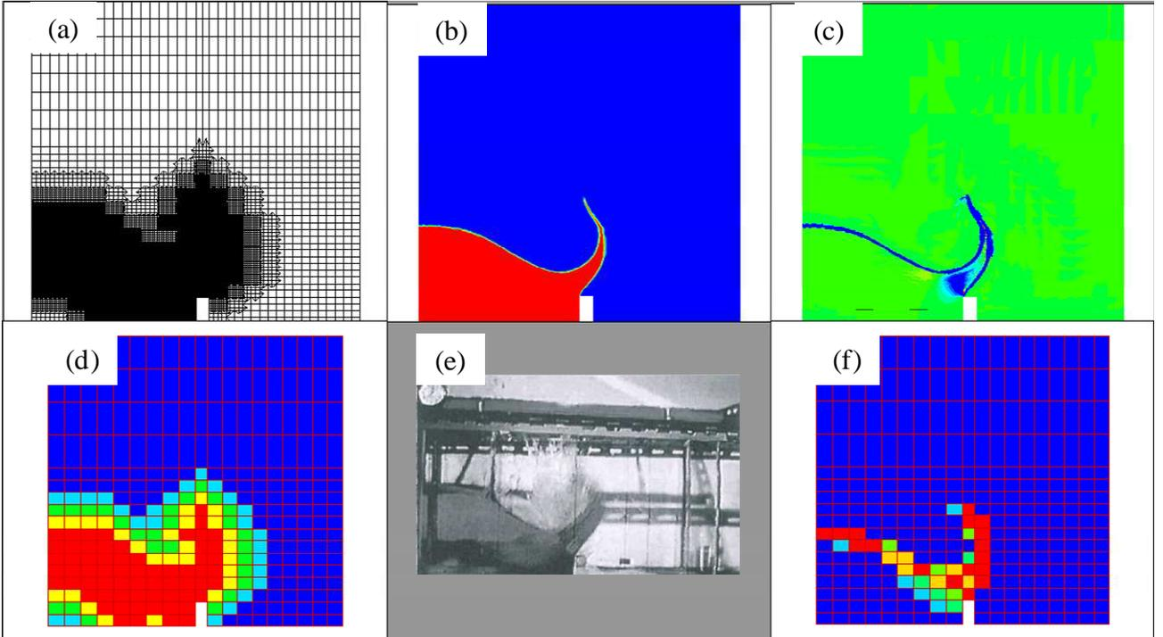
FIG. 2 – Dambreak with block remeshing at  $t=0.2s$ . (a) Mesh; (b) Density (air-blue, water-red); (c) Density of numerical entropy production (equation (2): green-zero, blue-negative values); (d) Mesh refinement level per block (1 to 5); (e) Experiment [16]; (f) Mesh refinement criterion per block.
