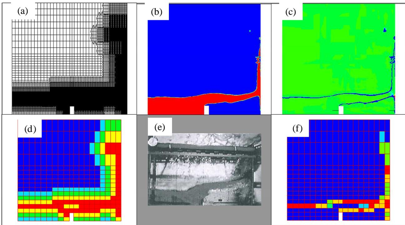
FIG. 3 – Dambreak with block remeshing at  $t=0.4s$ . (a) Mesh; (b) Density (air-blue, water-red); (c) Density of numerical entropy production (equation (2): green-zero, blue-negative values); (d) Mesh refinement level per block (0 to 4); (e) Experiment [16]; (f) Mesh refinement criterion per block.
