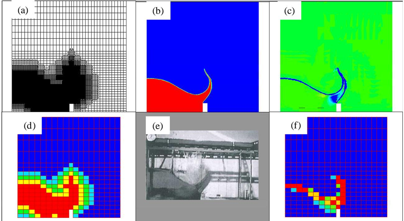
FIG. 2 – Dambreak with block remeshing at  $t=0.2s$ . (a) Mesh; (b) Density (air-blue, water-red); (c) Density of numerical entropy production (equation (2): green-zero, blue-negative values); (d) Mesh refinement level per block (0 to 4); (e) Experiment [16]; (f) Mesh refinement criterion per block.
