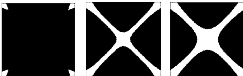
Fig. 1. Test 1. The computed coincidence set of the plastic zone for the bottom obstacle at the first (left), second (middle) and last (right) iteration.
