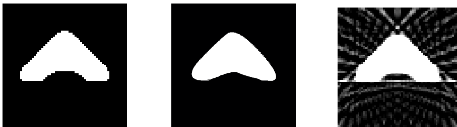
Fig. 7. Left: Original \Omega_2 . Center: NURBS-MCMC reconstruction. Right: FBP reconstruction. Both are using error 0.1%.
