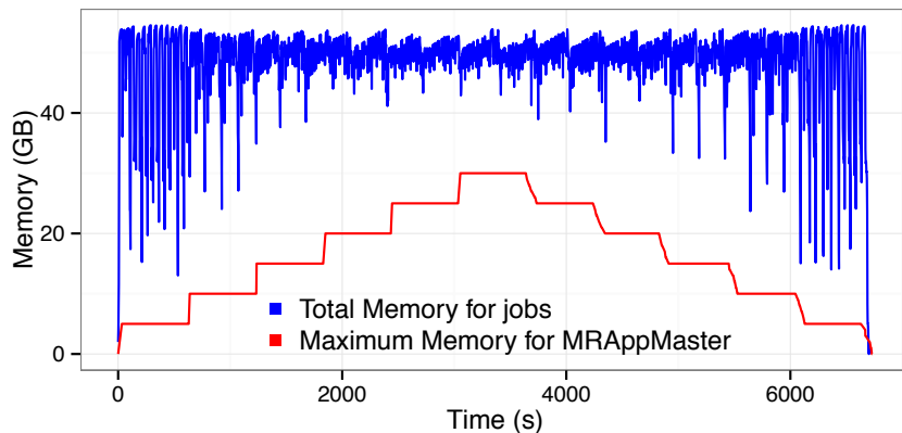
Fig. 4. Amplitude of memory drops depending on the MARP value.
