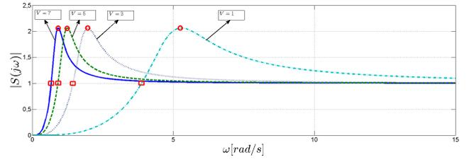
Fig. 3. Gain curve of the sensitivity function  $S$  (the sensitivity crossover frequency  $\omega_{sc}$  and the maximum sensitivity  $M_s$  are designated by  $\square$  and  $\circ$  correspondingly)
