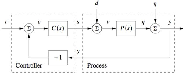
Fig. 1. Block diagram of a linear feedback loop
