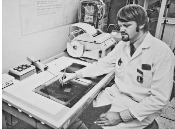
Fig. 2. The original man-machine radiotherapy interface with the Rho-Theta unit.
