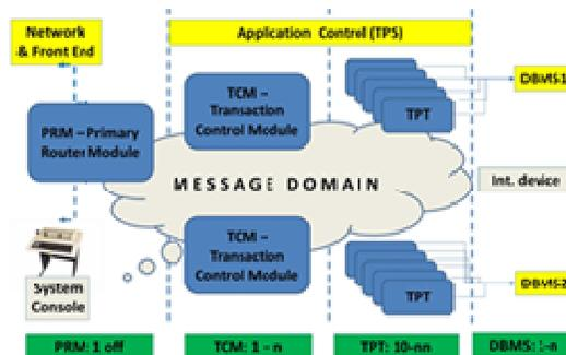
During normal operation on a full hardware configuration, the GTL system's network CPU contained the Network & Front End module, the next CPU contained the Application Control part, and the remaining two CPUs contained one SIBAS DBMS system each. For communication between the CPUs, a mini version of the previously mentioned Nordnet was used.
