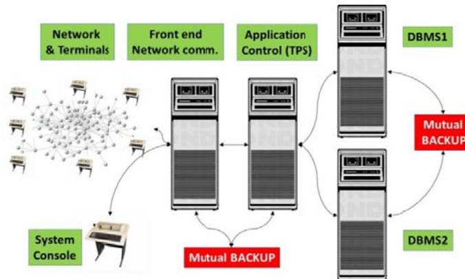
Two pairs of CPUs were mutual backup for each other. In normal operation one CPU interfaced to the NSB network, the next one contained all application programs, and the remaining two CPUs were both database machines. The database machines split the database between themselves in order to share the load, and trains would literally move between the database machines as they moved along the rail network in real life.
