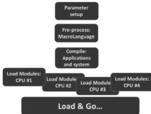
The output of the system builder was load images for each of the CPUs at hand, and the total system was initiated by loading the CPUs and typing the “initialize” command on the system console.
