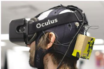
**Figure 2:** The Oculus Rift DK1 HMD<sup>a</sup> is combined with Neuroelectronics Enobio EEG cap<sup>b</sup> and OpenBCI amplifier<sup>c</sup> to both immerse and monitor user's brain activity.
