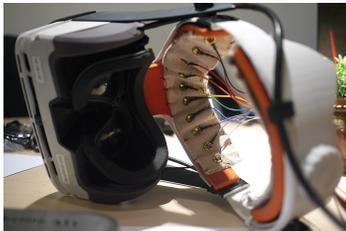
**Figure 3:** Prototype of a HMD device that directly embeds EEG electrodes – here a Vrvana Totem<sup>a</sup>. Picture © Alexandre Girardeau.
