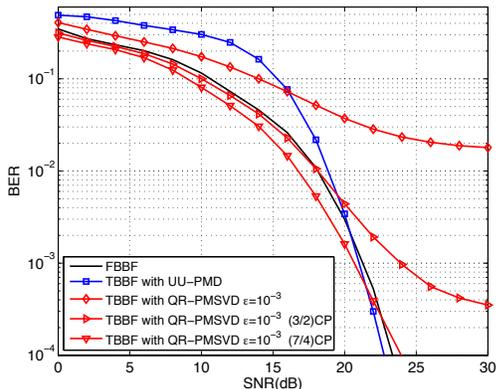
Fig. 4. BER comparison: FBBF, TBBF with UU-PMD and TBBF with QR-PMSVD in MIMO  $2 \times 2$  configuration. CP is extended to  $\frac{3}{2}$ CP then to  $\frac{7}{4}$ CP. The truncation parameter in the QR-PMSVD is set to  $\mu = 10^{-6}$ .
