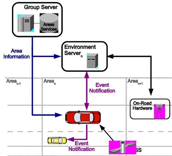
Figure 2: P2P/Cellular network overlay network for vehicular communications
